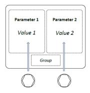
Parameter's value can be adjusted by rotating corresponding knob.
